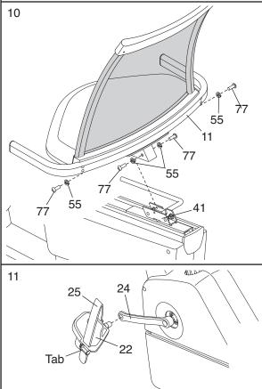
11. Identify the Left Pedal (22), which is marked with an "L." Using an adjustable wrench, firmly tighten the Left Pedal counterclockwise into the Left Crank Arm (24). Tighten the Right Pedal (not shown) clockwise into the Right Crank Arm (not shown). Important: Tighten both Pedals as firmly as possible. After using the exercise cycle for one week, retighten the Pedals.
